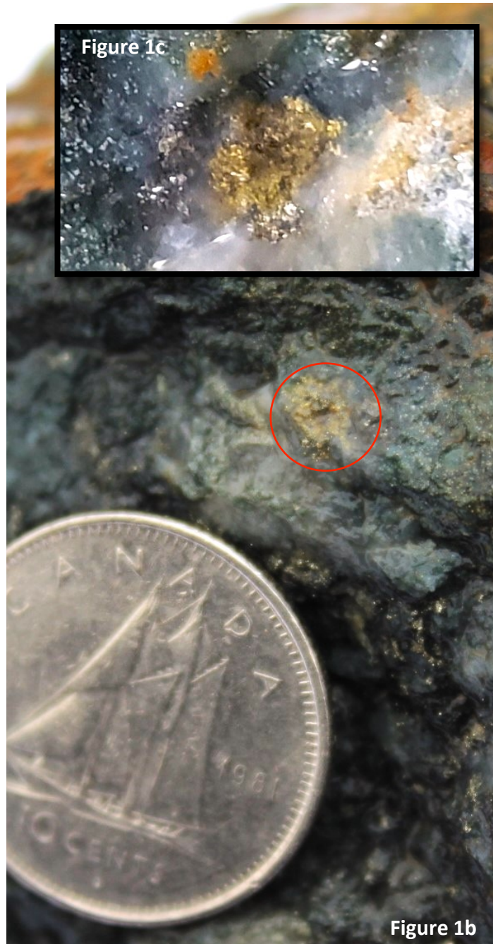
Visible Gold from the Conquest Zone. Photo 1a is from a cut surface; Photo 1b and 1c is from a broken surface.
