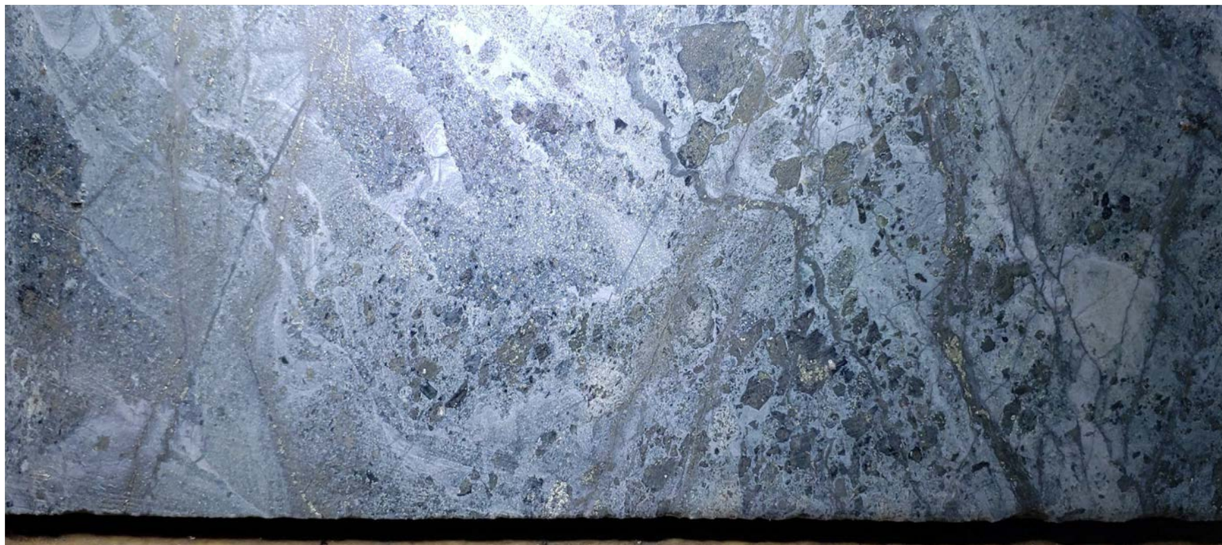
Root & cellar drill-hole 23RC-16 intersected 34.5 m of hydrothermal vent breccia grading 0.6 g/t Au
