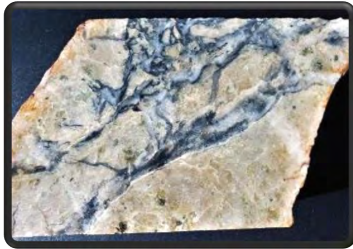
Quartz veins from Drop Zone hosting hessite (silver telluride). Sample assays up to 45 g/t Au, 1,365 g/t Ag and 700 ppm Te.
