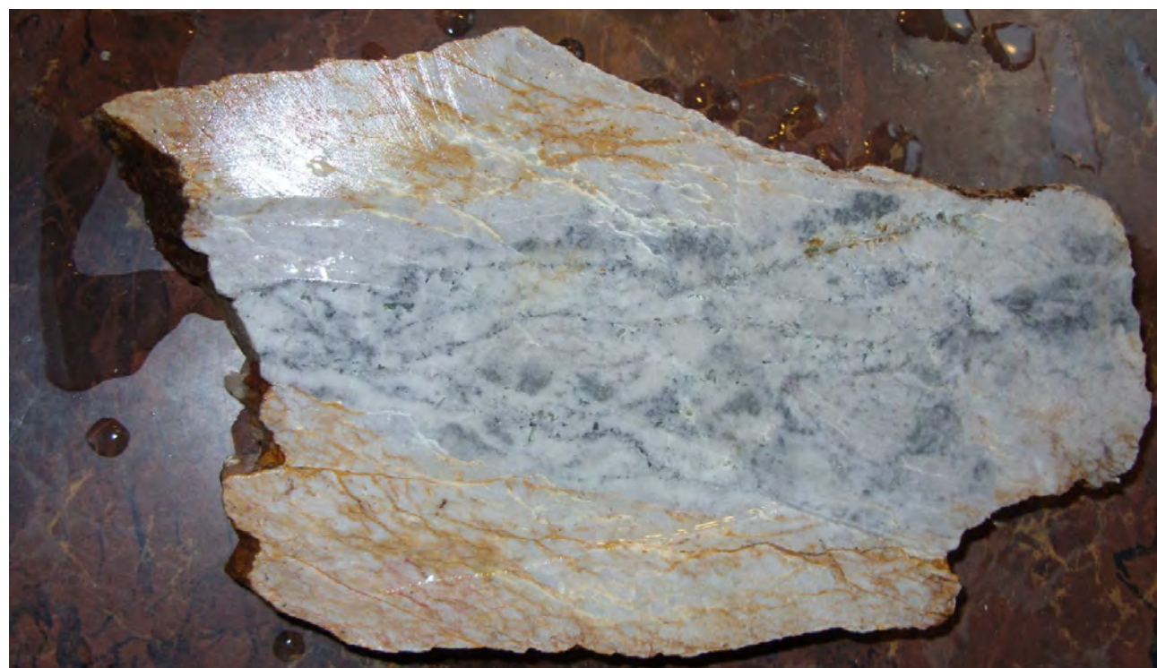
Quartz vein with up to 0.67 g/t Au, 0.65% Cu and anomalous Sb, As and Sn cutting quartz-sericite-pyrite alteration at "Fire" showing
